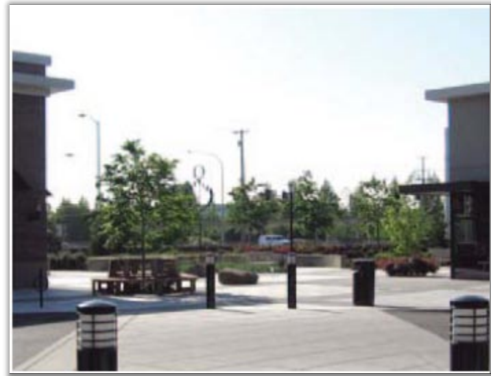
An example of a walkway with bollards that include light fixtures to clearly identify the pedestrian access.
