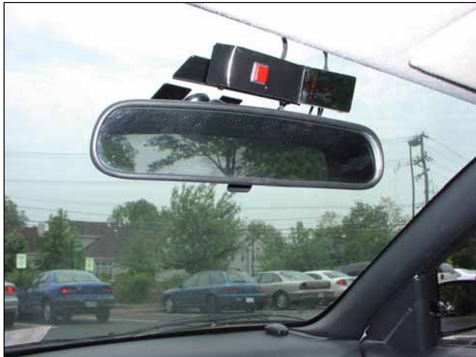
Figure 1.4. The incident pushbutton box mounted above the rear-view mirror. The portion on the right contains the driver-face/left-vehicle side camera hidden by a smoked plexiglass cover.
