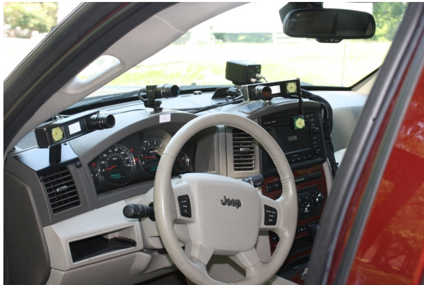
Figure 1. Eye tracking system camera placement.
