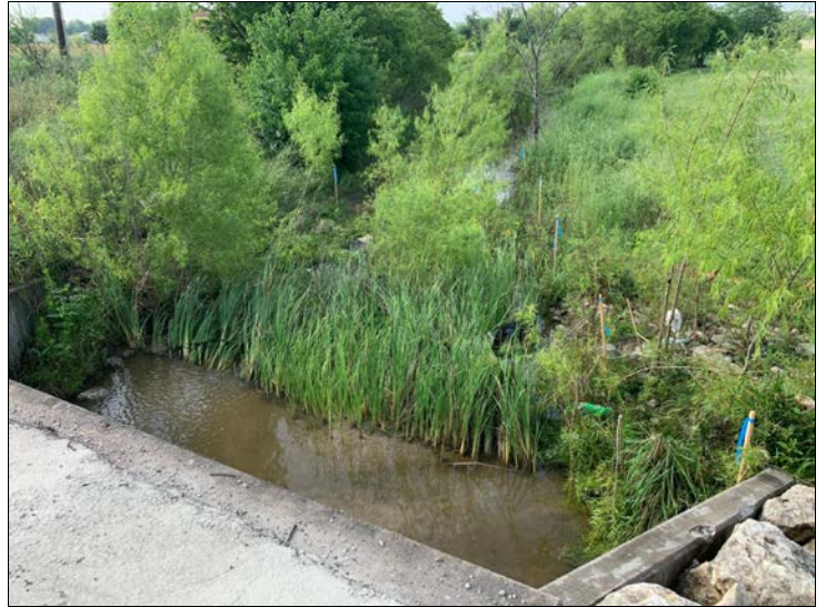
26. Looking south along intermittent Richmond Branch. Blue flagging denotes the extent of OHWM.
