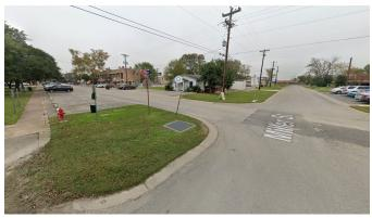
Example of Inaccessible conditions; lack of textured wheelchair ramps on each side of the street corner, and sidewalk is disconnected from street crossing, with no sidewalk on the other side of the road; lack of a clear crosswalk
