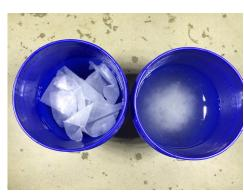
In a video demonstration, we showed how wipes (in bucket on the left) don't dissolve in water while regular toilet paper (in bucket on the right) does.
